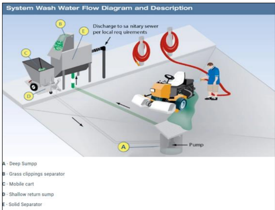
Figure 17. The ESD Waste 2 water equipment wash down system
